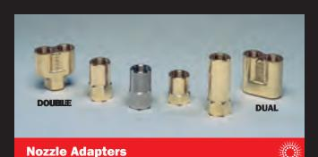
Single nozzle adapters ar e of fered in three sizes. Also available ar e both a double and dual adapter (single and two stage) which allow two nozzles to spray simultaneously or independently of each other . Standard construction is brass, but adapters made of Type 303 or Type 316 stainless steel ar e available on special or der. Available in either 1/8" or 1/4" NPT female connections. (See p. 5 for specifications.)
